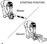
WARNING: When starting engine, hold the unit as illustrated. Do not set unit on any surface except a clean, hard area when starting engine or while engine is running. Debris such as gravel, sand, dust, grass, etc. could be picked up by the air intake and thrown out through the discharge opening, damaging the unit or property, or causing serious injury to bystanders or the operator.
